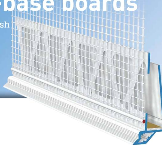
The **APU clip-on profile for plaster-base boards** (10 mm, 12 mm, 15 mm and 20 mm) is used horizontally in compound heat insulation systems, e.g., where plaster abuts with the cases of roller shutters or of external Venetian blinds.
