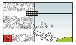
Holes to be cleaned of drilling dust.
