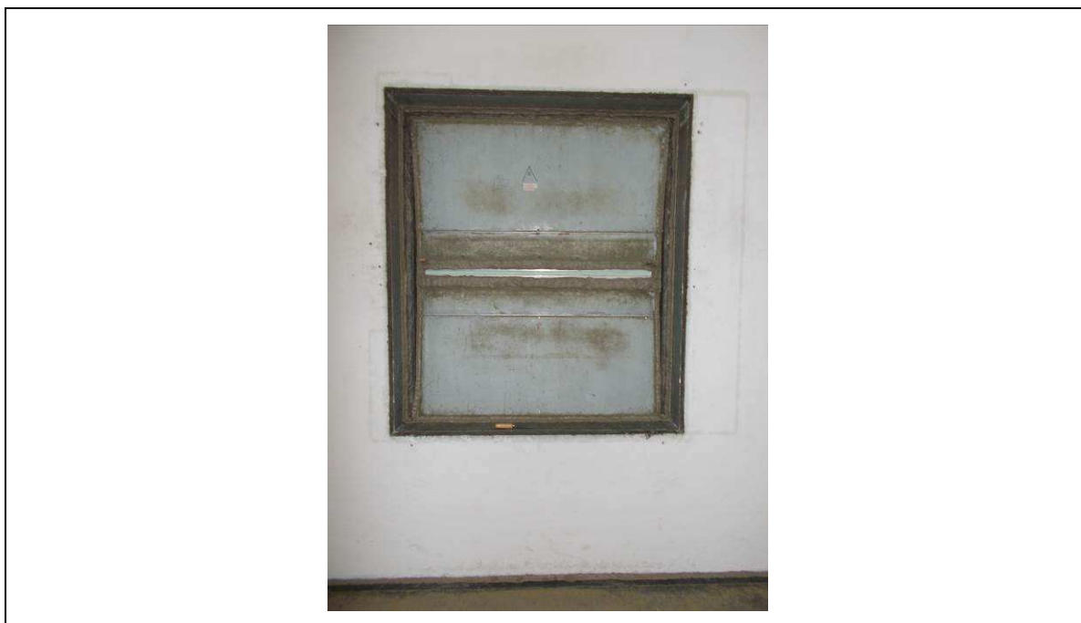
fig 3 Photo(s) of the mounted element, taken by ift Laboratory for Building Acoustics
