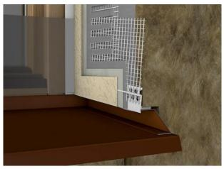
**Application:** PVC connecting sill side profile with exposed water drip edge and glass fibre mesh. Sill side profile with foam tape ensures expansion jointing of the plaster to the sill end in insulation systems ETICS. Drip edge provides safe water drain-off from the jambs and eliminates capillary rise under the insulating material. Glass fibre mesh meet the ETAG 004 requirements.
