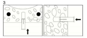
Fixing is not allowed for  $h_{ef} = 25$  mm and  $d_b < 35$  mm when a cavity is cut!
