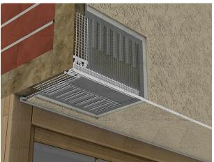
**Application:** Drip-nose profile PVC with glass fibre mesh. Drip-nose profile is used for finishing plaster in upper window and door reveals in insulation systems ETICS. Ensures dripping of water in vertical direction, due to which no return capillary action of water occurs. Profile protects against mechanical damage in insulation systems ETICS. Glass fibre mesh meet the ETAG 004 requirements.
