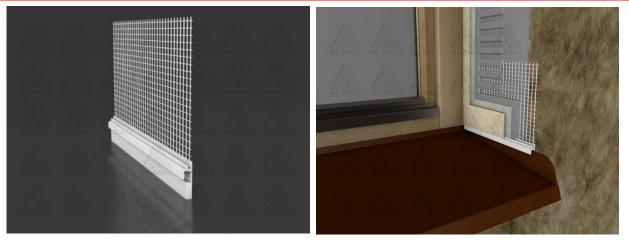
**Application:** PVC sill side connecton profile with glass fibre mesh. Sill side conncetion profile for sheet metal sill with a side bend, ensures a stable connection between sill and insulation system ETICS. It protects insulation system from mechanical damage and provides safe water drain-off from the system. Glass fibre mesh complying with ETAG 004.
