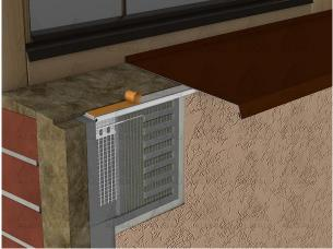
**Application:** Self-adhesive sill PVC profile  $90^{\circ} - 130^{\circ}$  with glass fibre mesh and self-adhesive foam tape is used to make safe, dense and flexible expansion jointing between the window sill and insulation system ETICS. Profile protects insulation system against mechanical damage and ensures water draining in vertical direction from the system. Glass fibre mesh meet the ETAG 004 requirements.
