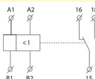
Always specify all reference name of current relay according to required range, for example PRI-51/5.
