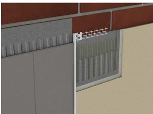
**Application:** Stop profile PVC with glass fibre mesh. Render stop profile is used for precise separation of coats of different structures and colors. It creates aesthetically connection between the plaster and the other construction elements in insulation systems ETICS. Appropriate for plasters with different thickness of laying – 3, 6, 10, 15 mm. Glass fibre mesh meet the ETAG 004 requirements.
