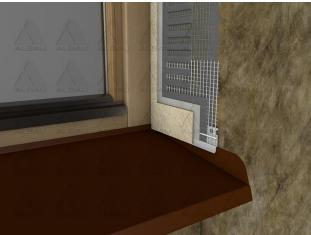
**Application:** PVC-UV and alkali resistant window sill profile with glass fibre mesh and invisible drip edge for flexible joining of window sill ending and thermal insulation system – ETICS (EWI). Suitable for connecting smaller metal flashings with plasters as well. It protects insulation system from mechanical damage and provides safe water drain-off from the system. Glass fibre mesh complying with ETAG 004.
