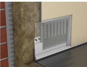
**Application** – EO-MC-20 is a metal sheet connection profile with fibre glass reinforcement mesh for expansion jointing of plumber's elements and facade in the point of connection to sheet metal in the contact insulation system – ETICS.
