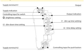
Recommendation for mounting: leave a gap of min. 0.5 module (approx. 9 mm) on side of the device to ensure better cooling of the device.
