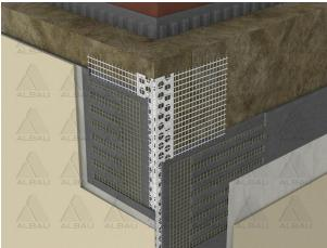
**Application:** universal PVC corner profile in roll with glass fibre mesh. The flexible roll of corner profile guarantees perfectly straight edges on all degrees of corners, especially around windows and doors where the system is prone to stress and strain. Minimizes cracks from occurring around openings in insulation system ETICS. Glass fibre mesh meet the ETAG 004 requirements.
