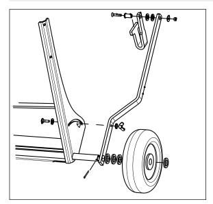
To replace the arms you have to remove the wheels and replace the two tub mounts (see adjacent illustration).
