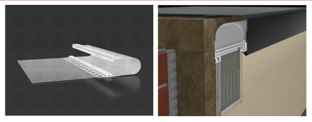
**Application:** EO-RE-20 closing profile with fiber-glass reinforcement mesh and rubber textile for closing the plaster at the roof edge and connecting it to the roof sheet metal in the contact insulation system – ETICS.
