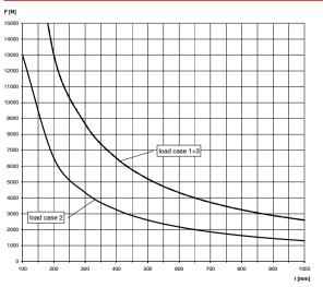
For the load curves, the permissible steel strain  $\delta_{adm.}$  = 160 N/mm and the maximum deflection under load 1/150 are not exceeded. Fixings and screw fastenings must be calculated accordingly.
