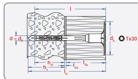
Determination of maximum thickness of insulation material:  $t_{\text{fix}} = L - t_{\text{tol}} - h_{\text{ef}}$  / Bepaling van de maximale dikte van isolatiemateriaal:  $t_{\text{fix}} = L - t_{\text{tol}} - h_{\text{ef}}$
