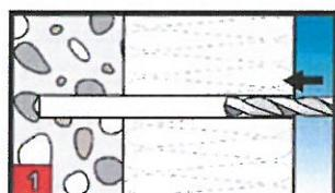
Create a hole about observation of the drill method according Annex C 1
